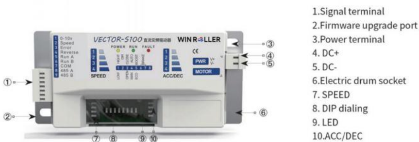
Layout of VECTOR-S100 DC Variable Frequency Motor Roller Driver
